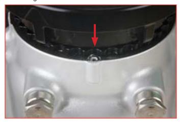
**Step 8)** Apply blue loc-tite to the 3/16" screw that was removed in step one then; thread it into the hole in the bottom of the casting until hand tight.
