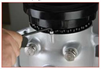
**Step 2)** Once the screw has been removed then the outlet can be unscrewed from the valve body by hand or by using a spanner wrench.
