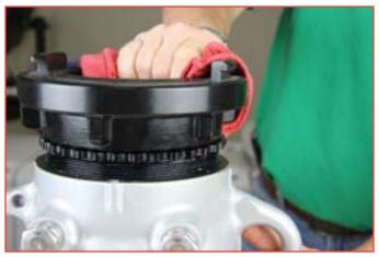
**Step 3)** Remove the valve seat from the unit using the pointed pick. When the outlet was removed from the unit the o-ring either stayed in the unit or came out with the outlet. Locate and remove.
