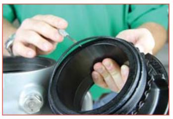
**Step 4)** Wipe away any debris and inspect the leading edge of the valve plunger for damage. If damage is clearly evident the plunger may need to be replaced.
