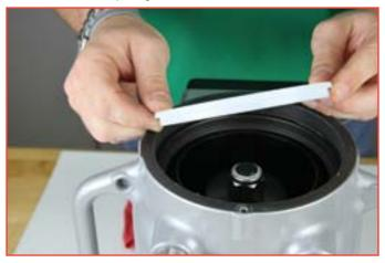
**Step 6)** Using the grease included in the kit, grease the o-ring grooves where indicated in the photo. Install the o-ring on the outlet. (Do not install the o-ring in the unit first as the o-ring will likely be damaged during re-assembly.) Grease over the o-ring and the threads of the outlet fitting.
