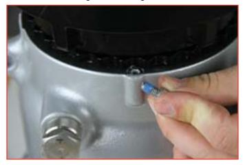
**Step 9)** Leak test – Hook the valve to the appropriate appliance either a hydrant or a hose. Before pressurizing the unit; insure that the valve is in the closed position. Do not attach hose to the outlet of the appliance, this will allow for visual inspection of the seat. Pressurize the unit to approximately 50 lbs. Inspect the seat and outlet area for leaks. If no leaks are present shut down the water supply source and bleed the pressure.
