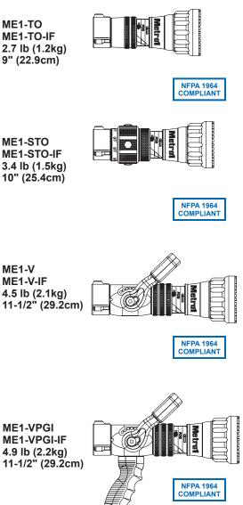
ME1-TO - METRO 1 TIP 1.5" NH (38mm) Fixed gallonage tip with 14 flow / pressure choices. Includes flush without shutting down, molded rubber teeth for full-fill "power fog" pattern, "Gasket Grabber" inlet screen. Lightweight hardcoat anodized aluminum for maximum resistance to corrosion and wear. Tip does not shut off and must be used with a separate valve or valved playpipe. 1.5" NH (38mm) rigid rocker lug coupling is standard
