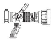
**ME2-2VPGI** - METRO 2 W/GRIP 2.5" NH - Fixed gallonage nozzle with 10 flow and pressure choices. The METRO 2 includes a pressure-assisted flush without shutting down, ball valve shut-off and molded rubber teeth for full-fill "power fog" pattern. Lightweight hardcoat anodized aluminum for maximum resistance to corrosion and wear. Pistol grip is mounted below the valve. 2.5" NH (65mm) full-time swivel rocker lug coupling is standard. **IJ = 1.5" NPSH Threads**
