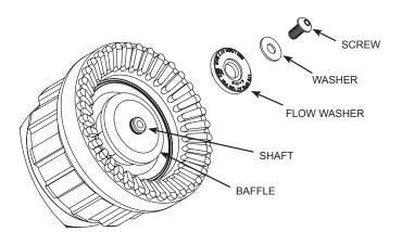
The flow washers are marked with various flow settings. Change flow washer to the desired setting. The nozzle will flow the indicated amount when the pressure at the nozzle is at the indicated level.
