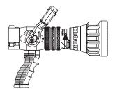
**ME2-VPGI** - METRO 2 W/GRIP 1.5" NH - Fixed gallonage nozzle with 10 flow and pressure choices. The METRO 2 includes a pressure-assisted flush without shutting down, ball valve shut-off and molded rubber teeth for full-fill "power fog" pattern. Lightweight hardcoat anodized aluminum for maximum resistance to corrosion and wear. Pistol grip is mounted below the valve. 1.5" NH (38mm) full-time swivel rocker lug coupling is standard.
