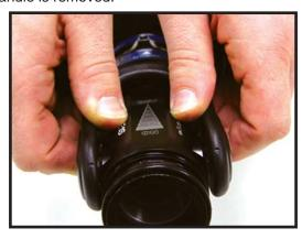
**Step 6)** Use your finger to pull out the stainless steel slide valve. Two o-rings seal the slide valve, there will be some resistance when it is pulled out.
