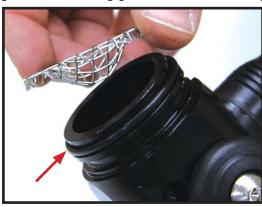
**Step 20)** Install the debris screen over the valve body so the concave portion faces down over the valve body. Next, lightly and evenly press the coupling down onto the valve body. Pay close attention that the o-ring does not get pushed out of place or pinched.
