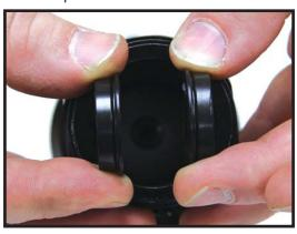
**Step 14)** Lightly grease the outside circumference of the slider with the grease provided in the kit. Install the slider with the chamfered edge facing the valve plug. Use caution when installing the slider that it does not pull the valve discs out of place. Push the slider in until it contacts the valve plug then pull back about 3/8".
