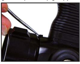
**Step 2)** Holding the nozzle over a container with the port plug hole facing down rotate the coupling until all the ball bearings fall out. 33 balls retain the coupling. Once all the ball bearings have been removed pull off the coupling, debris screen, and o-ring.
