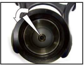
**Step 19)** Included with the kit is a new o-ring to seal the coupling to valve body connection. Lightly grease this o-ring. Install this o-ring on the valve body as shown. Also, lightly grease the ball ring groove on the valve body.
