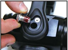
**Step 18)** With the valve handle held in the closed position, using the 3/16" Allen wrench back the valve plug out (unscrew) unit it makes firm contact with the slider. Once contact is made with the slider, open the valve handle part way and unscrew the valve plug 10 degrees. This will set the proper tension between the valve plug and slider.
