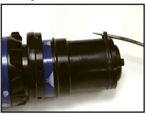
**Step 5)** With the grease included in the kit lightly grease the o-ring groove in the barrel, install the new o-ring, then lightly grease over the o-ring.
