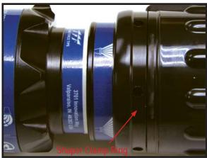
**Step 2)** Using the TG500 or 3/16" pin spanner, insert the pin in one of the six holes in the shaper clamp ring. While holding the shaper by hand or with a strap wrench loosen the clamp ring counterclockwise. This may require a quick initial jolt to break the ring free
