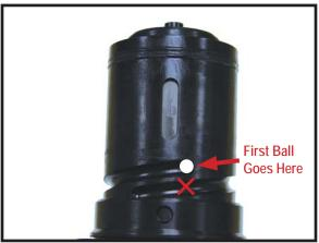
**Step 7)** With the nozzle still on end slide the new shaper over the barrel. Continue to slide it on until the shaper covers the Torlon balls.
