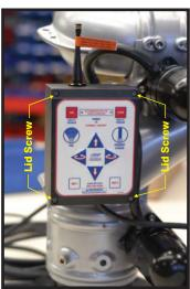
1) Turn off power and remove lid from monitor control box. Unscrew the lid screws but do not remove screws completely from lid. Be careful to open lid slowly as lid is connected to communication board by a flat cable.
