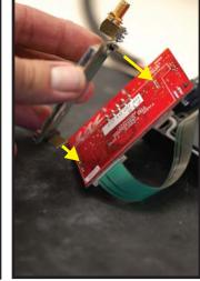
5) Plug radio board into 6) Attach antenna connector to communication board. Be careful to line up pins.
