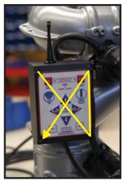
10) Tighten lid screws equally in a criss-cross pattern.
