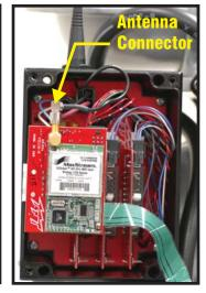
radio board with the cable in the orientation. Note, in some RC monitors, cable tie may need to be cut to attach antenna.
