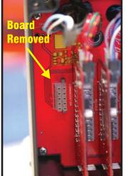
4) Remove the small communication board on the far left. Pull board straight out.
