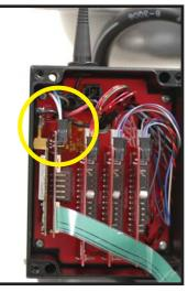
7) Plug communication 8) Insert connector with blue & board/radio board into main white wires into communication board. Press down to seat board. securely.
