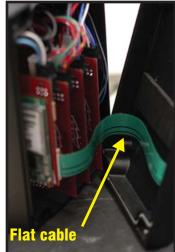
9) Replace lid onto box. Be sure to guide flat cable down across motor boards and to not pinch any wires between lid and box.
