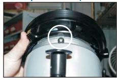
**Step #9B)** If desired, install lock out ball. Apply a small amount of grease to the ball pocket to help retain the ball in position. Push coupling on completely. If lock out ball is being used, note alignment.
