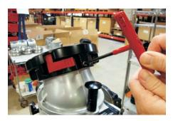
Step #9A) If a rigid/locked-out connection is desired. Push coupling onto unit. Align threaded hole in coupling with lock-out detail in unit. Apply Loctite® 242 to lock out screw. Thread screw into coupling until it touches the bottom of the lockout detail. Do not over tighten – this will result in leaks.
