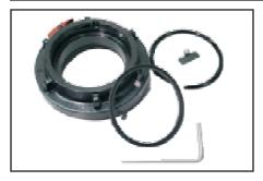
Items required: Replacement coupling, port plug or port cover, Dow 112 grease, pointed pin/seal pick, pliers, polymer strip removal tool THA401, cup seal, 7/32" allen wrench, Loctite® 242 and lockout ball. All items are supplied in our coupling replacement kits.
