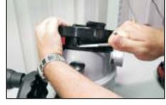
**Step #3**) Insert THA401 into port as shown, with hook side up. Engage with polymer ring.
