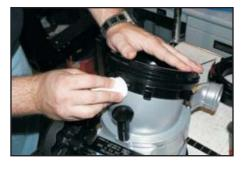
**Step #12)** Use a degreaser to clean the area of the port is the cover type is used. Use short end of the THA401 to assist in the installation of the port plug. Install till flush.
