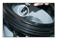
Step #10) Insert polymer ring into the port with the blunt end first.
