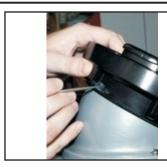
**Step #1)** Using the seal pick or pointed pin, remove the port plug or port cover, which is used to cover the access port to the polymer ring.
