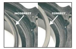
**Step #8)** Install cup seal as shown above. Apply grease to the cup seal only.
