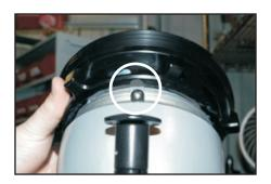
**Step #10)** Push coupling on completely. If lock out ball is being used, note alignment.
