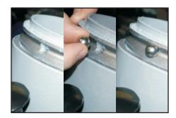
**Step #9)** If desired, install lock out ball. Apply a small amount of grease to the ball pocket to help retain the ball in position.
