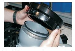
**Step#6)** Remove coupling, cup seal and lock out ball if present.
