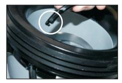
**Step #11)** Insert polymer ring into the port with the blunt end first.
