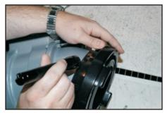
**Step #2)** If the coupling swivels, rotate till the end on the polymer ring can be seen through the access port. The ring can also be moved with the seal pick if required.
