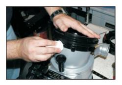
**Step #13)** Use a degreaser to clean the area of the port is the cover type is used. Use short end of the THA401 to assist in the installation of the port plug. Install till
