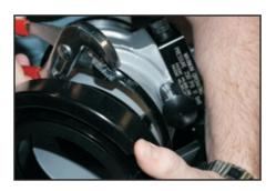
**Step #5)** Once the strip is exposed by several inches you may remove using pliers.
