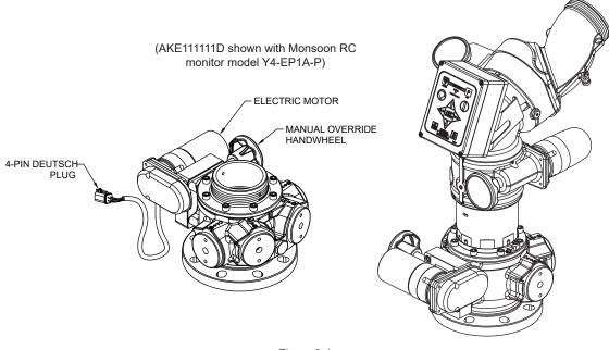
Figure 3.4c VUM WITH ELECTRIC REMOTE CONTROL ( VUM RC )
