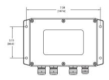
Figure 4.4.1 Valve Interface Enclosure Mounting Hole Dimensions
