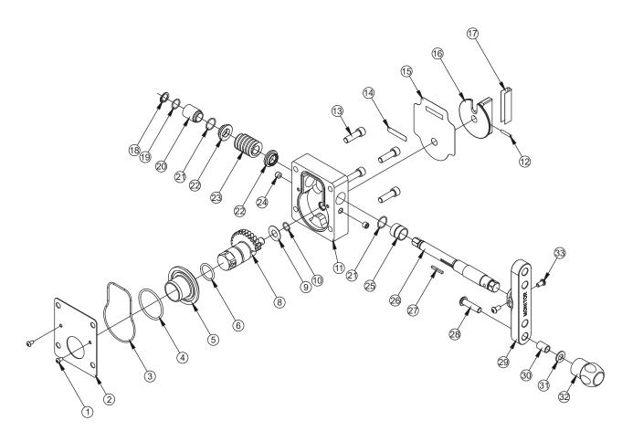
Figure 6.0b Exploded View of Worm Drive Gearbox
