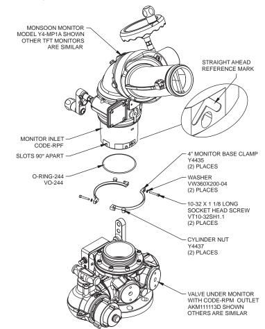
Figure 4.3d CODE-RPM DIRECT CONNECTION WITH TWO PIECE CLAMPS
