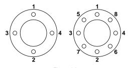
Figure 4.2 Flange Bolt Tightening Sequence
