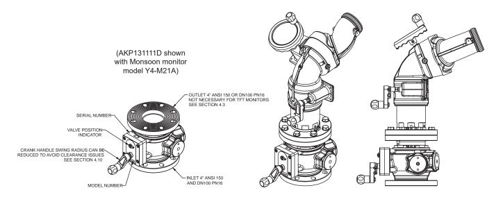
Figure 3.4b VUM WITH PARALLEL DRIVE GEARBOX
