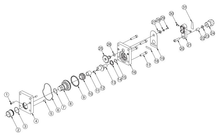
Figure 6.0c Exploded View of Parallel Drive Gearbox
