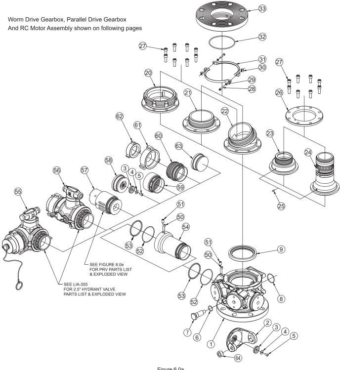
Figure 6.0a Exploded View Without Gearbox
