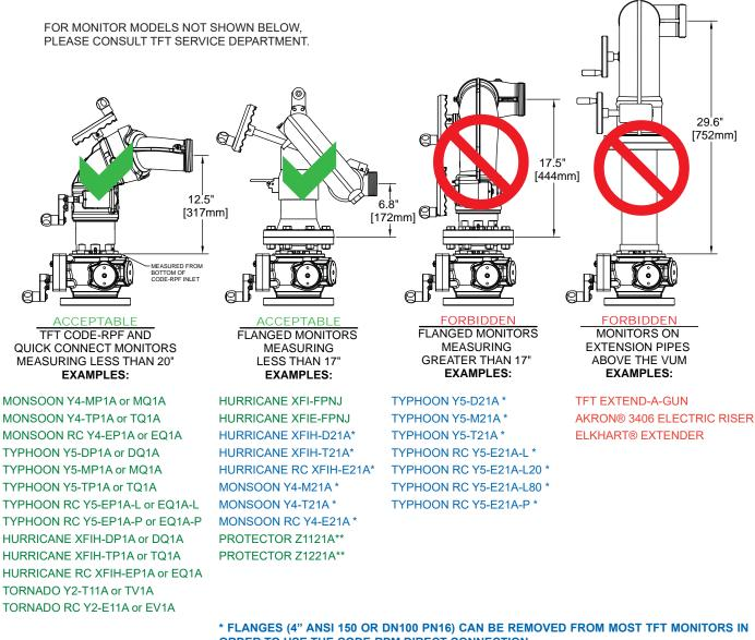
ORDER TO USE THE CODE-RPM DIRECT CONNECTION. \*\*THESE PROTECTOR MONITORS WITH 19.2" (48.8 cm) OUTLET HEIGHT ARE ACCEPTABLE UP TO 1250 GPM AT 250 PSI (4800 L/MIN AT 17 BAR).
