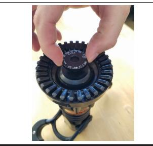
STEP 5 - Install the appropriate flow calibration disc onto the shaft with the desired calibration showing.
