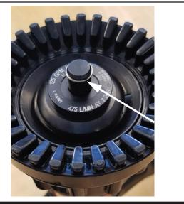
STEP 2 - Use the point of a knife, pick, or small screwdriver to pry the end of the retaining ring out of its groove. http://tft.com/metro/remove
