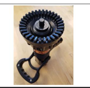
STEP 3 - Pull ring out of the groove by unwinding in a clockwise direction. Use care to avoid deforming the groove in the shaft. Do not reuse the old ring. Caution – ends of ring can be sharp.
