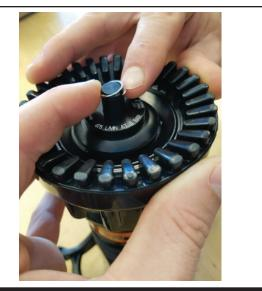
STEP 6 - Separate the coils of the new Spirolox® retaining ring and insert end into groove. Wind Spirolox® retaining ring in a counter-clockwise direction into groove. http://tft.com/metro/install
