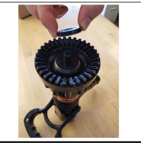
STEP 4 - Remove the old flow calibration disc from the shaft, leaving the baffle installed.
