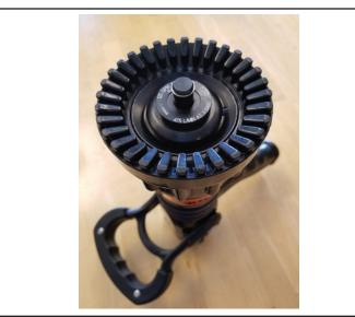
STEP 1 - Set nozzle to FLUSH position. Push baffle and flow calibration disc down to expose the Spirolox® retaining ring.
