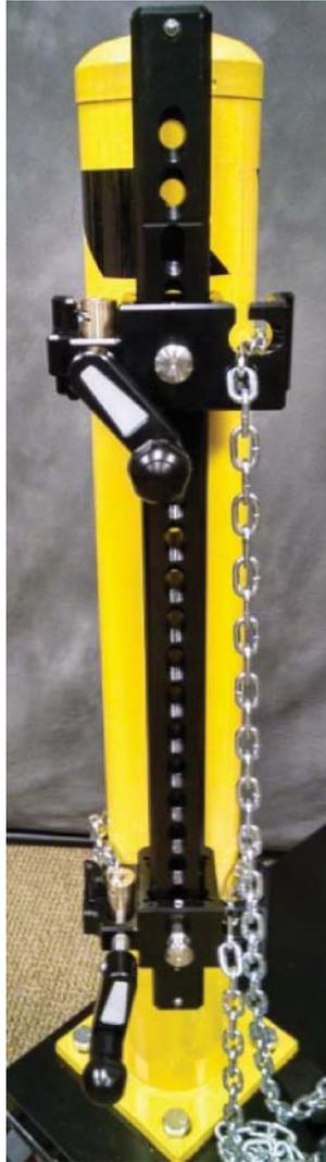
Figure 2.29 Install the other chain block
