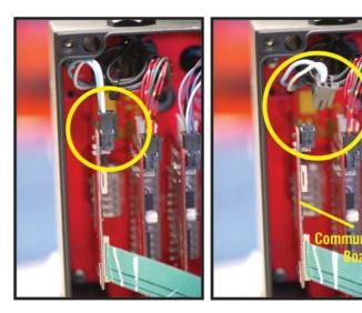
1) Turn off power and remove lid from monitor control box. 2) Locate connector with blue Unscrew the lid screws but do not remove screws completely from lid. Be careful to open lid slowly as lid is connected to communication board by a flat cable.
