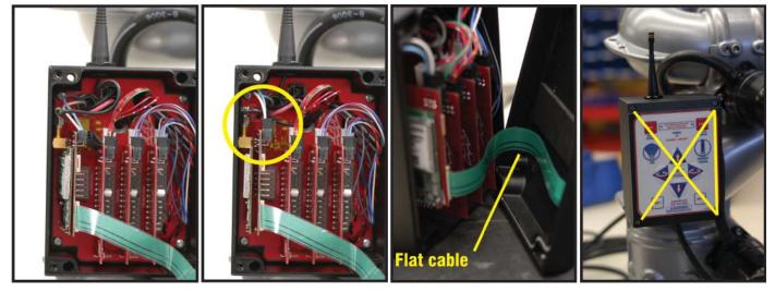
7) Plug communication board/ radio board into main board. Press down to seat securely.
