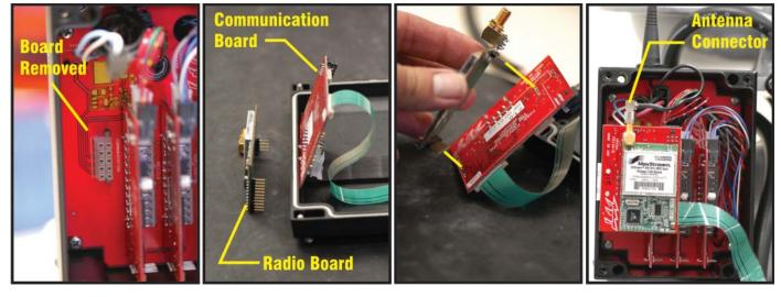
4) small Remove the communication board on the far left. Pull board straight out.
