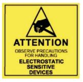
Observe precautions for handling Electrostatic Sensitive Devices. Be sure to touch unpainted, exposed metal on monitor or firetruck before removing and handling circuit boards.
