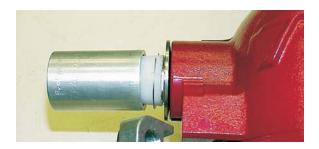
**18)** Install Smalley Ring to retain Belleville spring on trunnion.
