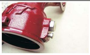
19) Install stationary trunnion into bell section with red Loctite. Turn trunnion in until tight making sure that it engages the threads in the ball.
