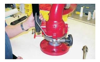
**28)** Align 'hexes' and push valve handle onto trunnion while engaging slide link in hole on bell.
