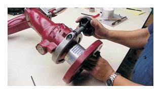
2) Remove knob assembly. Remove cotter pin from end of locking nut. Remove locking nut, castle nut, washer and knob.
