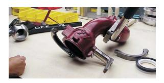
5) Using 1-1/8" inch socket (or wrench) remove the stationary trunnion from the right side of the housing.
