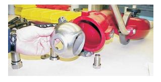
**9)** Grasp ball with hex hole on the bottom and circular opening on the right.
