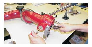
7) Using the T-handle hex wrench, remove washer, plug and screw. These parts are not reused with the valve parts.
