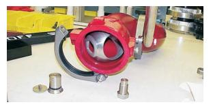
**10)** Insert the ball into the bell housing rotating the hex hole to your left so the circular hole is facing you.
