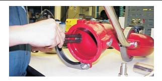
6) Remove the Plug from the other trunnion hole with a allen wrench and a pin spanner (the holes for the pin spanner are on the end of the Plug that is inside of the Monitor).
