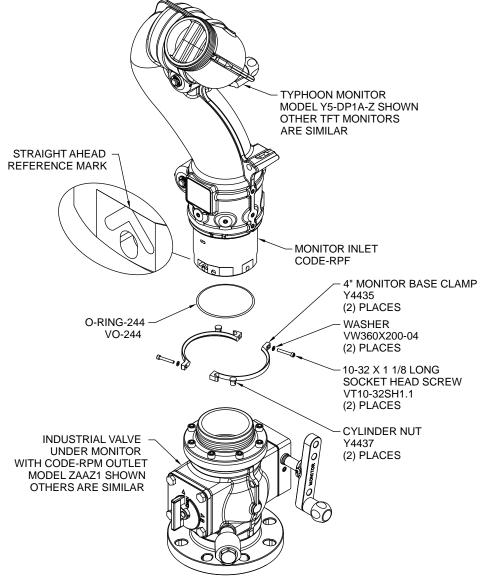
Figure 9: CODE-RPM Direct Connection
