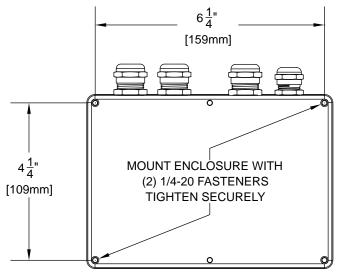
Figure 11: Valve Interface Enclosure Mounting Hole Dimensions
