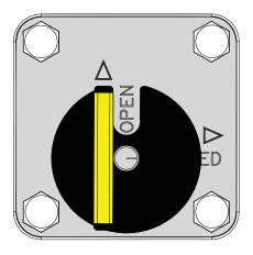
Figure 15: Valve Position Indicators
