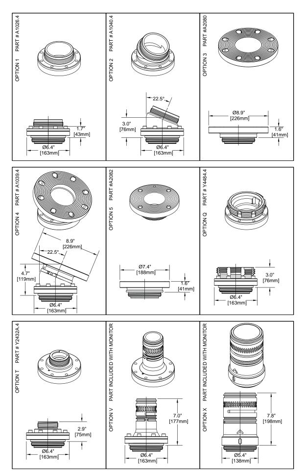
Figure 5: Side "B" Monitor Outlet Options
