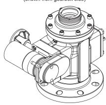
model ZAAZT-RC or ZASZT-RC with 2.5" NH quick connect for Tornado monitor (shown from gearbox side)
