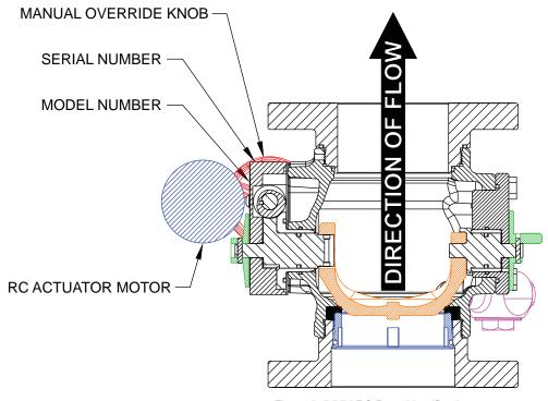
Figure 2: IVUM RC Parts Identification
