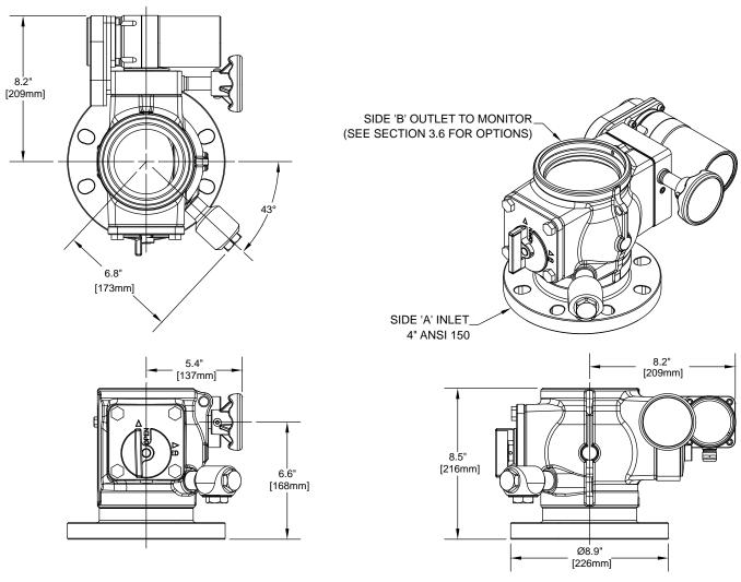
Figure 4: IVUM RC dimensions without monitor outlet
