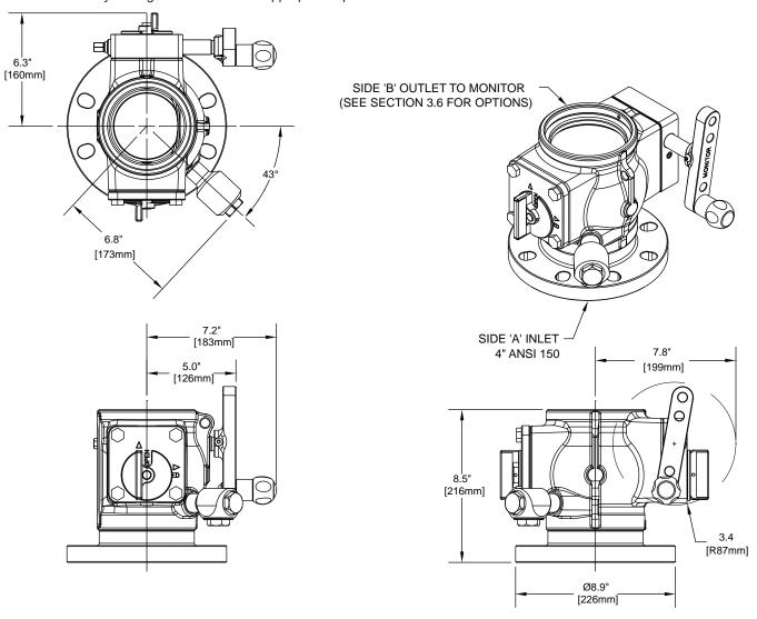
Figure 3: IVUM dimensions without monitor outlet
