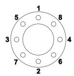
Figure 6: Flange Bolt Tightening Sequence
