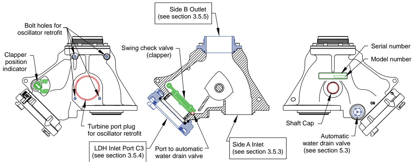
Figure 3.4: Parts Identification and Intended Orientation
