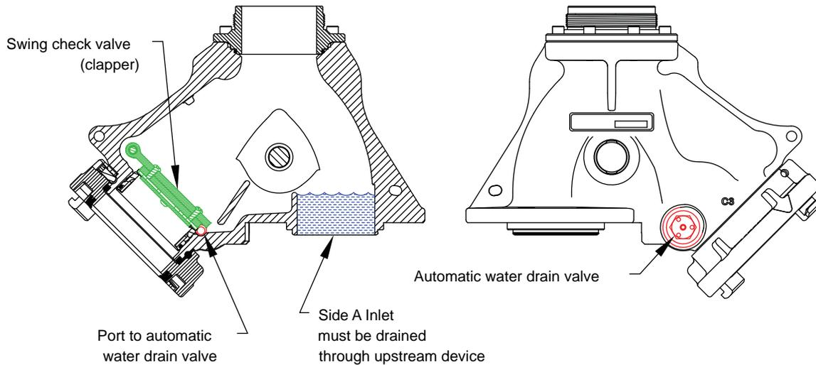
Figure 5.3: Draining Residual Water
