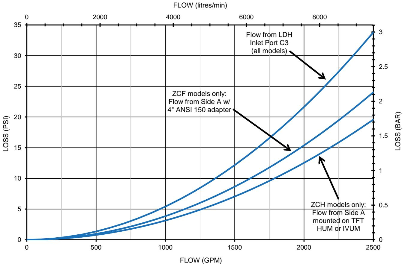
Figure 7.0: Flow rate versus pressure loss curves
