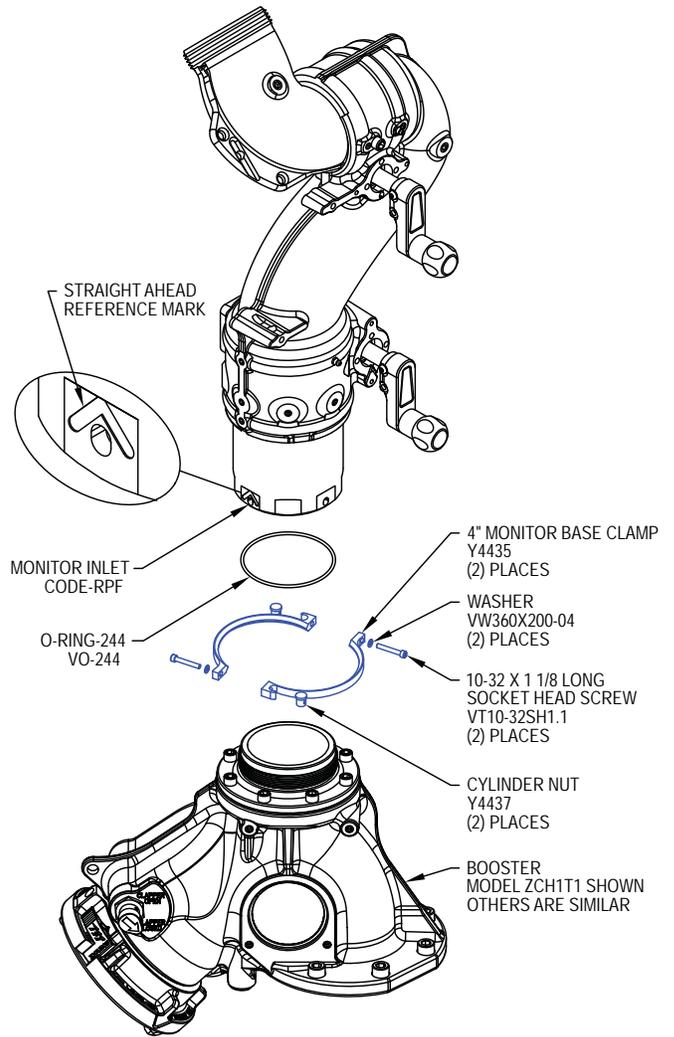
Figure 4.3.1: CODE-RPM Direct Connection
