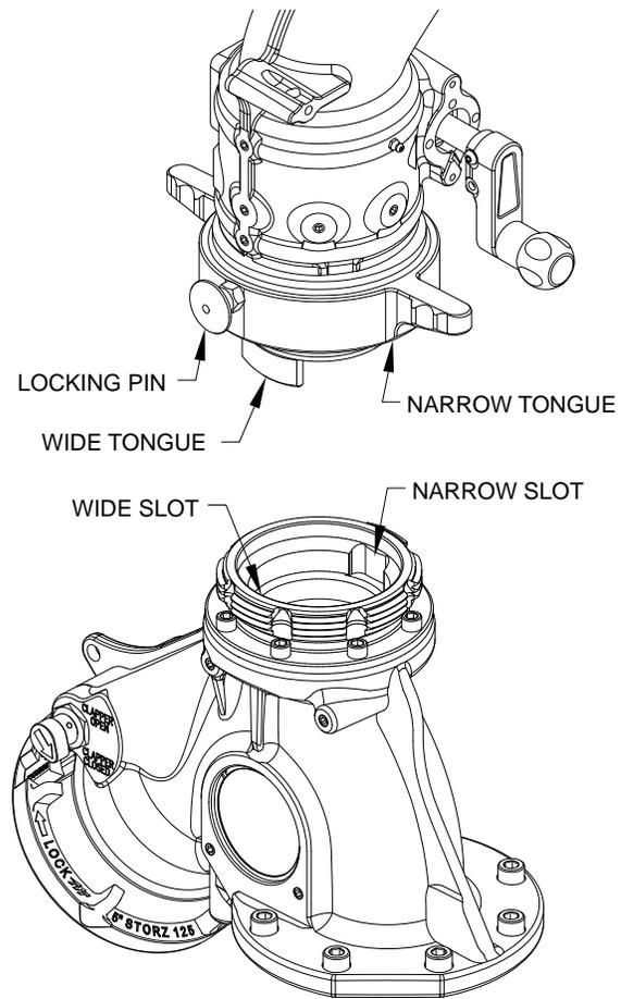
Figure 4.3.3: Quick Connect Installation
