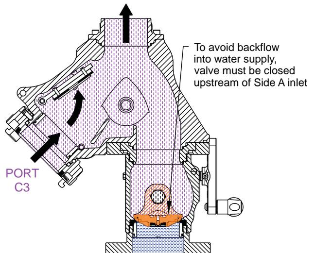
Figure 5.2.2b: Booster mounted on IVUM or other valve
