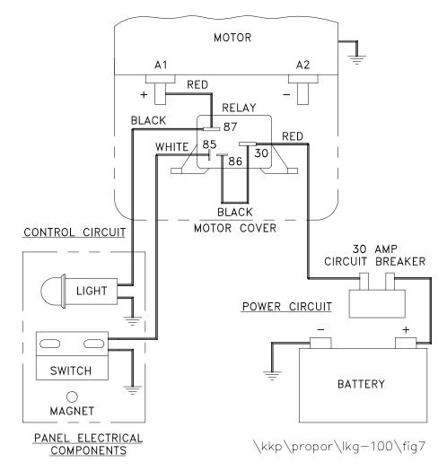
FIGURE 7 - TRUCK MOUNT - MOTOR WIRING DIAGRAM
