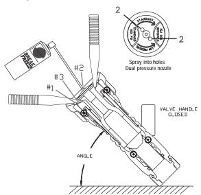
While holding nozzle at the angle, wait 30 seconds for the lubricant to penetrate into the clearances. Cycle the valve handle and rotate the shaper from straight stream to full flush several times, and then proceed to the next section.
