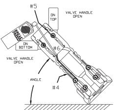
While holding nozzle at the angle, wait 30 seconds, then cycle the valve handle several times. Rotate the pattern control from straight stream to full flush several times. The pattern control should move freely and easily. The barrel cone should move forward to within 1/16" of the baffle before the shaper reaches straight stream position. Wipe off excess lubricant.
