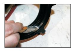
9) Grease plastic strip groove and sealing area in new coupling using Dow 112.
