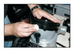
15) Clean dirt, debris, and grease off of coupling.
