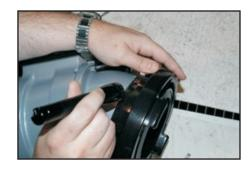
2) If coupling is not locked-out, swivel coupling around until the end of the plastic strip can be seen.
