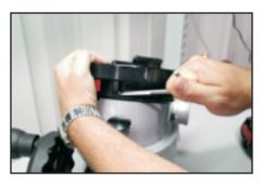
3) Insert puller tool (available from TFT Part Number: THA401) into coupling as shown and hook the end of the plastic strip
