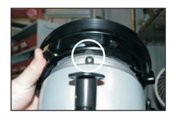
12) Push new coupling on until it stops.Note alignment of lockout ball detail.
