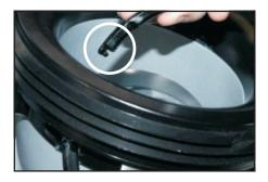
13) Push new plastic strip into port. **Note: Hooked end goes in last.**
