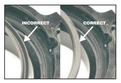
10) Grease cup seal, if used, with Dow 112 and install into coupling with sealing lips down (away from you).
