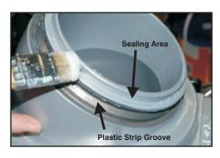
8) Re-grease plastic strip groove and sealing area using Dow 112.
